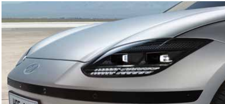
Parametric pixel lights (Projection type full-LED headlamps) 點陣式組合燈 (投射式全LED頭燈)
