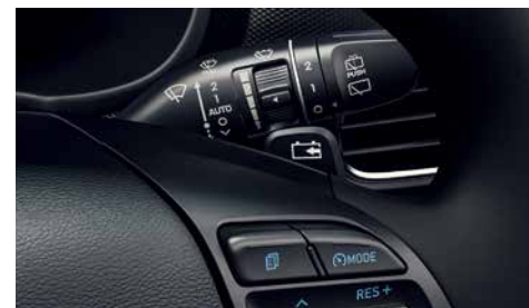
Paddle shifter (Regenerative braking control) 軛盤撥片 (能量回收制動控制)
