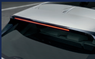
空氣力學延長尾翼 Extended Aerodynamic Rear Spoiler
