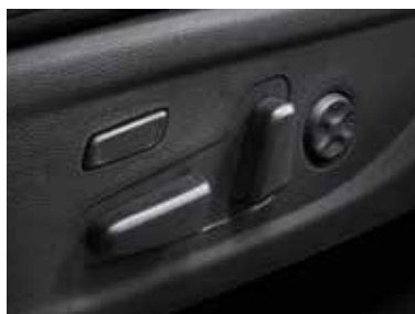
Driver's 14-way Power Seat 司機席14向電動調控
