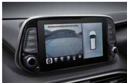
Surround View Monitor (SVM) A multi-camera system provides a 360-degree view around the vehicle to assist the driver in parking situations.
