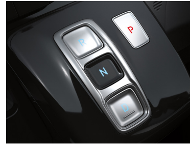
按鍵式換檔按鈕 Shift-by-wire automatic transmission
