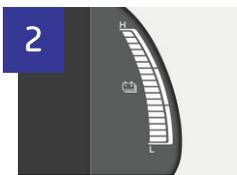
2 : SOC(high voltage battery) Indicator indicates the charge state of the high voltage battery.
