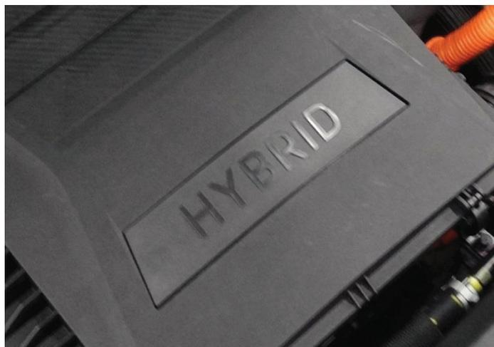
Additionally, there are orange colored high-voltage electrical cables in the engine compartment.
