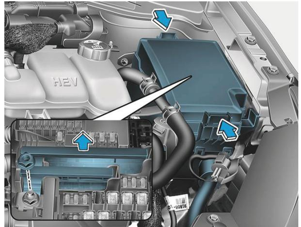
3. In the event the vehicle cannot be disabled using the “Power” START/STOP Button, pull the IG1, IG2 fuses or relays from the engine compartment room fuse box. If the IG fuses cannot be located, pull out all the fuses and relays in the fuse box.
