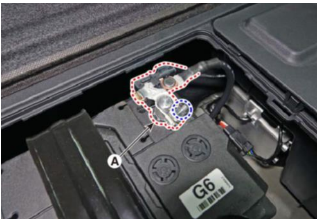
3-3. Turn the ignition switch OFF and disconnect the auxiliary 12V battery negative (-) terminal (A).
