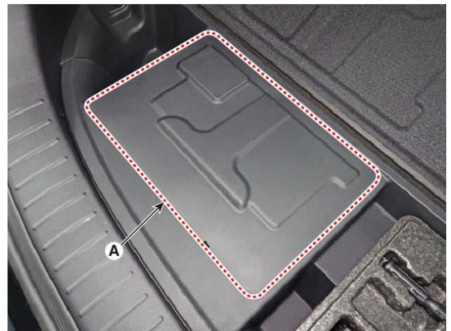
3-2. Remove the 12V battery service cover (A).
