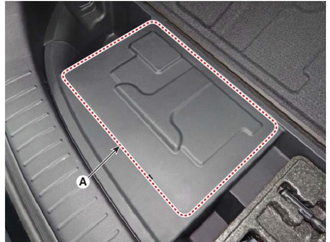
4-2. Remove the 12V battery service cover (A).
