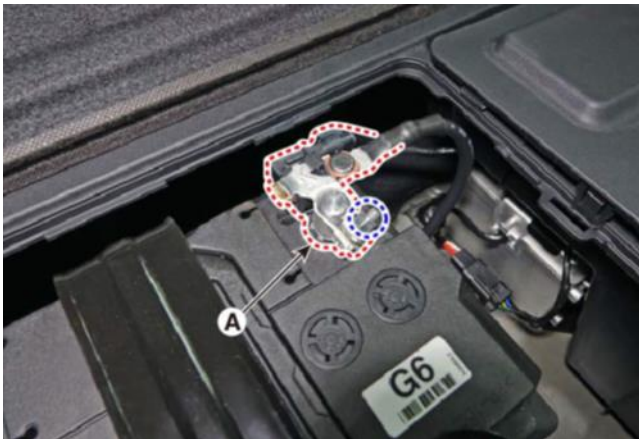
4-3. Turn the ignition switch OFF and disconnect the auxiliary 12V battery negative (-) terminal (A).
